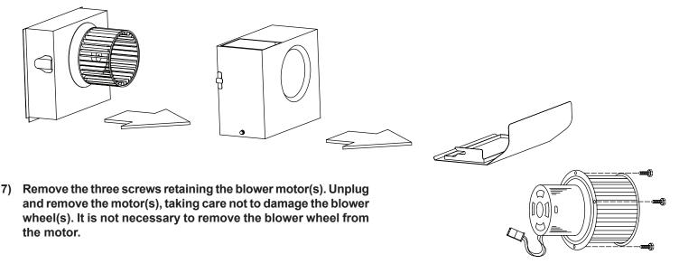
Warning: Make sure power is off and locked at the service disconnecting means on the service panel during installation.
